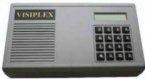
The VS1810 offers a simple and powerful alarm inputs monitoring capabilities and provides a serial interface to paging encoders or any other device that requires serial communication input.
